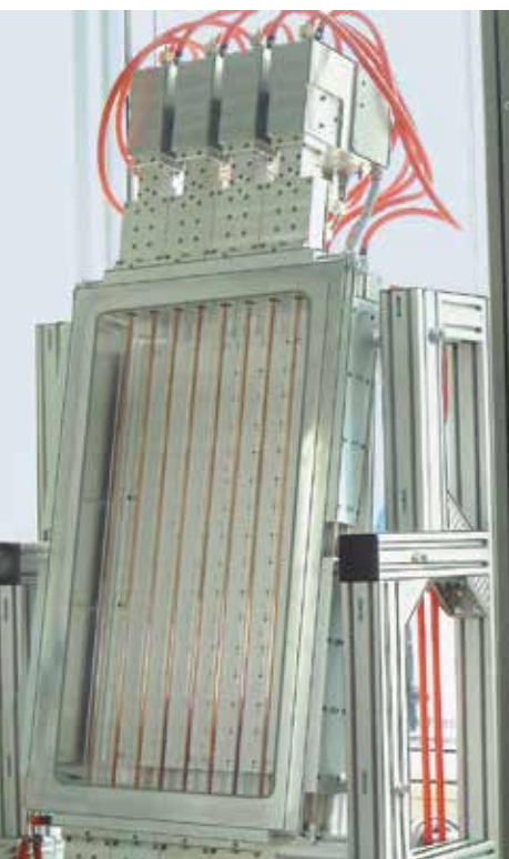
The plasma array (on the left) produces a planar plasma and a homogeneous plasma density. The specimen holder on the right contains the 50 x 100 m 2 test samples © Fraunhofer ICT
