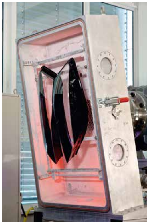
The plasma array (on the left) produces a planar plasma and a homogeneous plasma density. The specimen holder on the right contains the 50 x 100 m 2 test samples © Fraunhofer ICT
